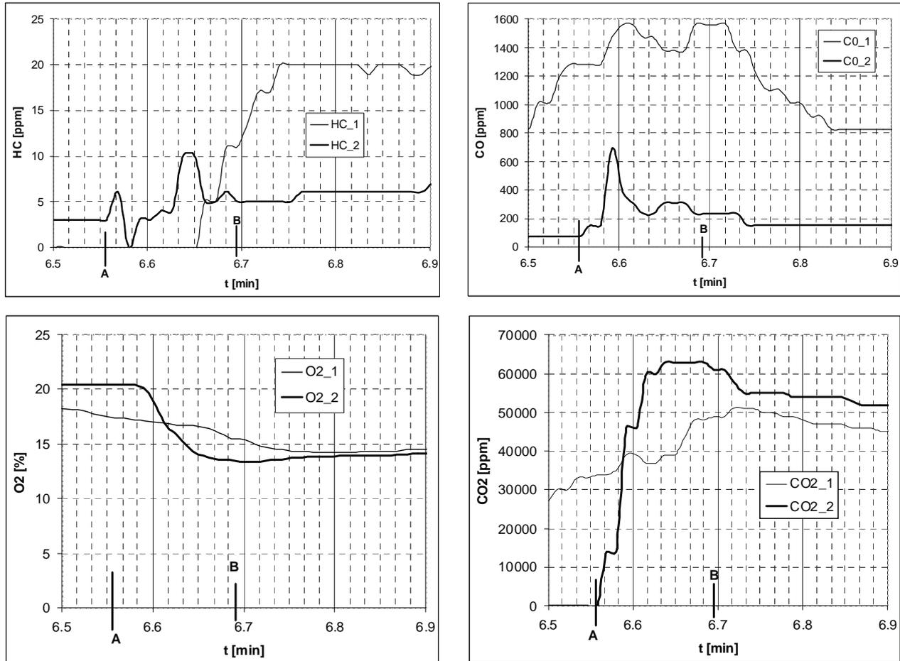
Fig. 3. Concentration of hydrocarbons HC, carbon oxide CO, oxygen  $O_2$  and carbon dioxide  $CO_2$  on the upstream and downstream side of the Pt/Pd catalytic reactor (initially heated up to  $400^\circ C$ ) during the 4CT90 engine start-up and at ambient temperature of  $-7^\circ C$
