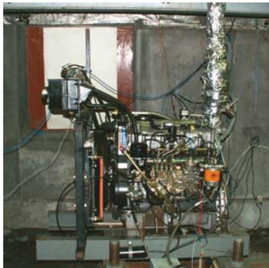
*Fig. 1. Testing station with 4CT90 engine and insulated catalytic reactor in the climate chamber*
