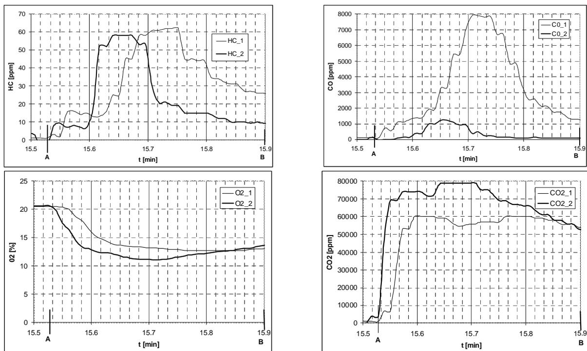
Fig. 5. Concentration of hydrocarbons HC, carbon oxide CO, oxygen O<sub>2</sub> and carbon dioxide CO<sub>2</sub> on the upstream and downstream side of the Pt/Pd catalytic reactor (initially heated up to 400°C) during the 4CT90 engine start-up and at ambient temperature of  $-15^{\circ}\text{C}$
