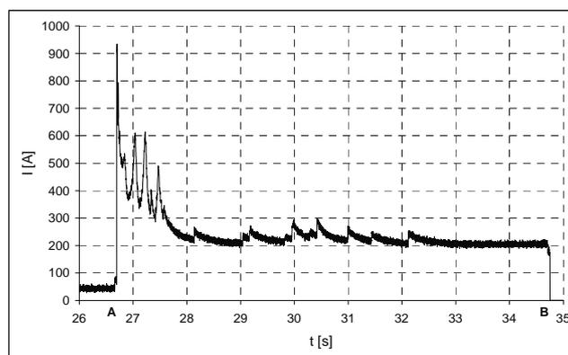
Fig. 4. A course of current intensity drawn by the starter during the 4CT90 engine start-up at ambient temperature of  $-7^\circ C$
