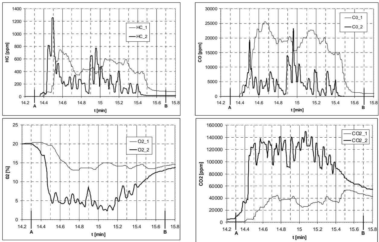
Fig. 7. Concentration of hydrocarbons HC, carbon oxide CO, oxygen  $\text{O}_2$  and carbon dioxide  $\text{CO}_2$  on the upstream and downstream side of the Pt/Pd catalytic reactor (initially heated up to  $400^{\circ}\text{C}$ ) during the 4CT90 engine start-up and at ambient temperature of  $-20^{\circ}\text{C}$
