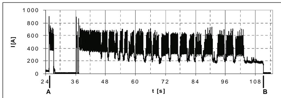
Fig. 8. A course of current intensity drawn by the starter during the 4CT90 engine start-up at ambient temperature of  $-20^{\circ}\text{C}$
